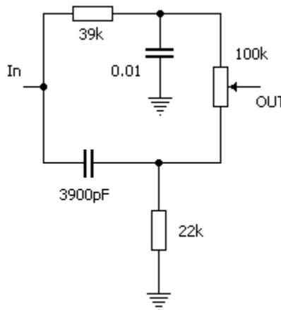
This is the classic tone stack from the Big Muff distortion pedal. It is basically a pair of filters whose output is combined through the 100k mix pot. The 39k/.01 filter passes only low frequencies and attenuates the highs. The 3900pF/22k filter does the opposite; it passes highs and filters out the lows. The 100k pot blends together the signal from each filter and therefore acts as a tone control.
