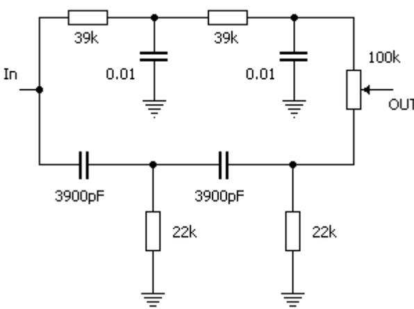
We can alter the response of the tone control in an interesting manner merely by including an additional set of R-C filters to the control. The frequency rolloff is essentially doubled and sounds outside the filter band are rejected more effectively. This can be a musically useful modification to the basic tone control.
