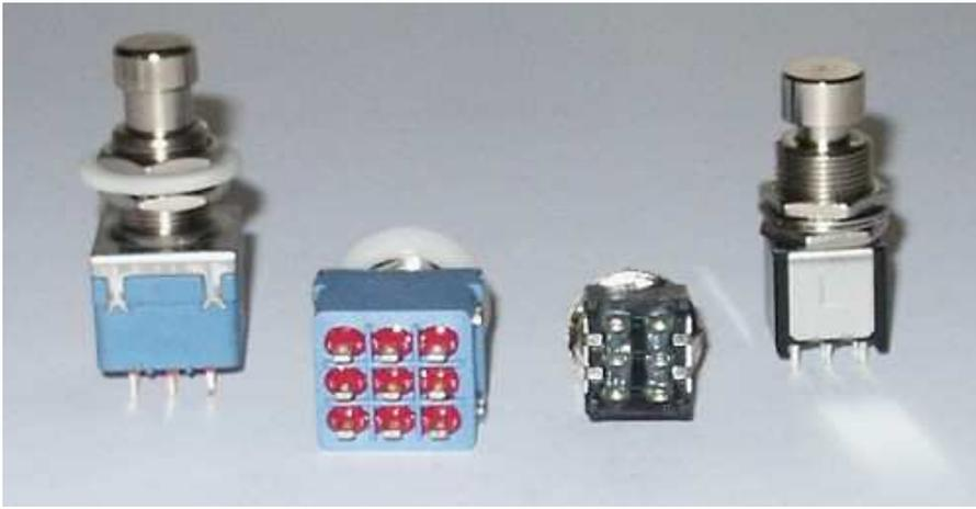
For comparison, a 3PDT and DPDT are shown in this photo. The 3PDT is the pair of switches on the left and the DPDT is the smaller pair on the right. The DPDT is Mouser part number 107-SF12020F-L or they are available at [Small Bear Electronics](#).
